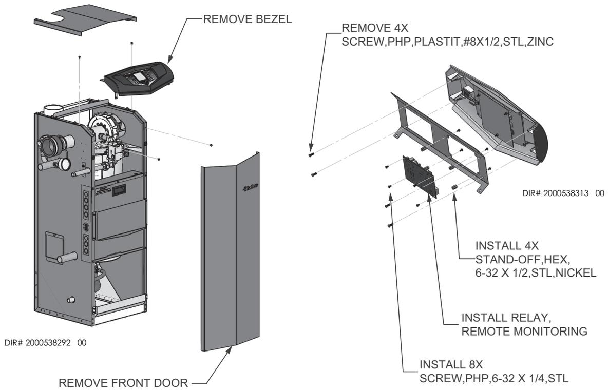
Figure 2-2E\_Install AW CON·X·US Board
